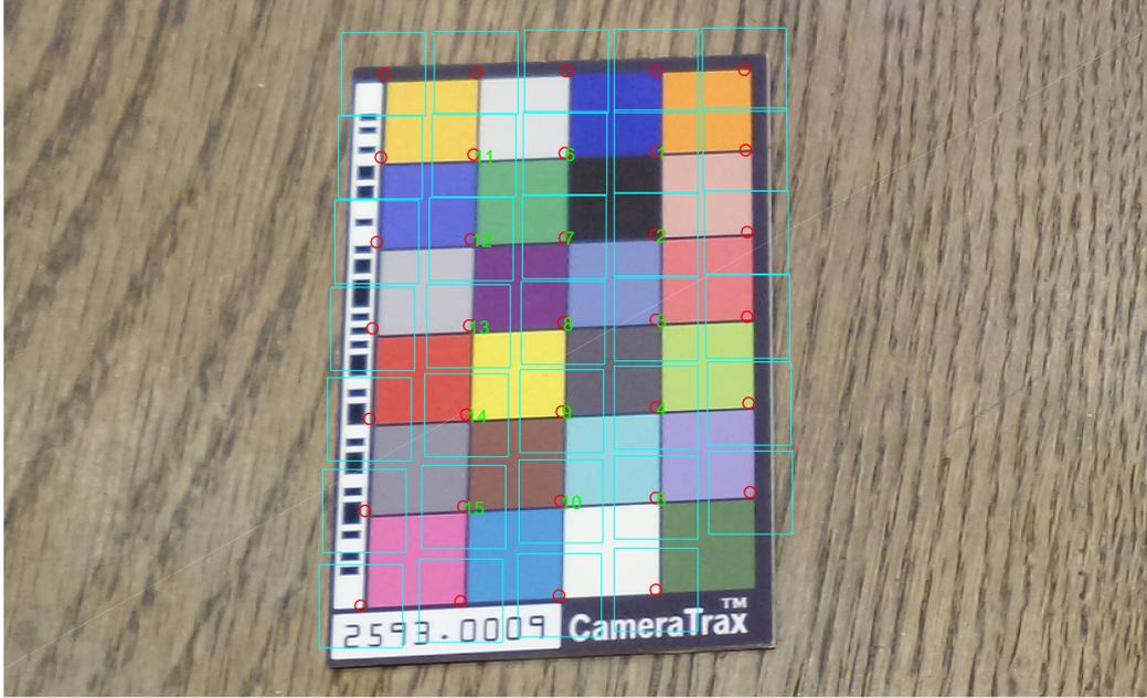
Figure 9: The feature vector is computed for all lattice points and matched to known feature vectors of the inner color patches of the color checker card's specification
