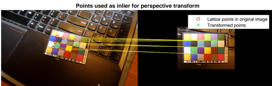
Figure 13: Image before and after computing the perspective transform Only some lattice coordinates are used for the transform.
