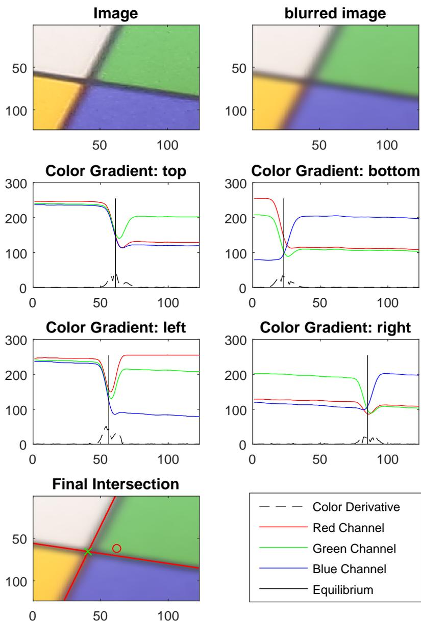
Figure 10: Example of a single fine adjustment step. Based on an initial starting point (red), we consider an excerpt from the image and blur it. Then the color derivatives are calculated for the outermost top/bottom/left and right segments of this excerpt, which yields to an approximation for the intersection point (green)
