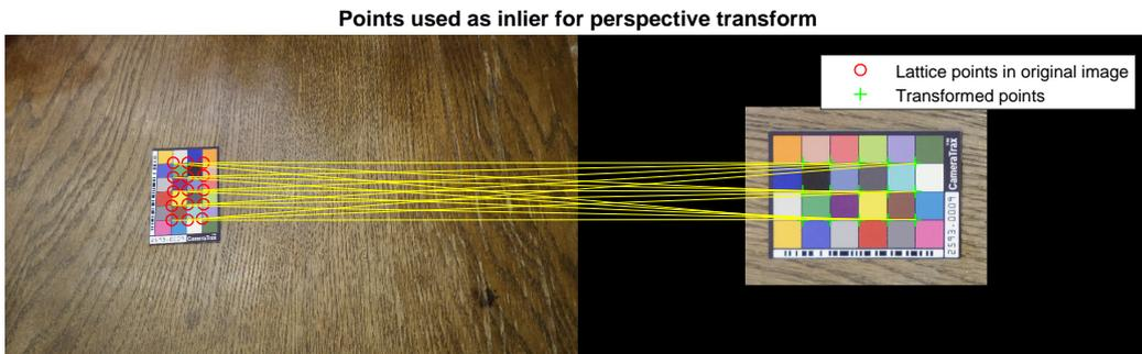
Figure 12: Image before and after computing the perspective transform. All lattice coordinates are used as inliers.
