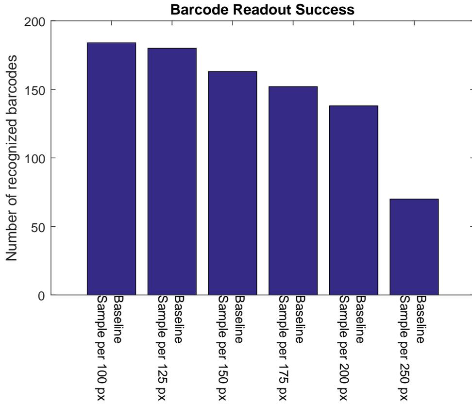
Figure 17: Barcode Readout Success for different baseline variant
