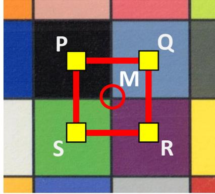
Figure 8: The feature vector is computed using the averaged color of four points within the quadratic surrounding of the point  $M$ .
