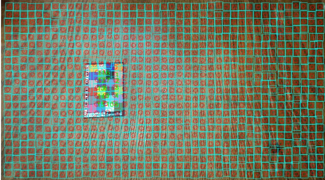
Figure 15: Equidistant Variant without lattice detection: Uniform equidistant samples across the entire length of the image. First the fine adjustment step is applied and then the point labelling is performed
