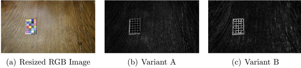
Figure 6: Original image (a) and different edgemap variants (b-c)
