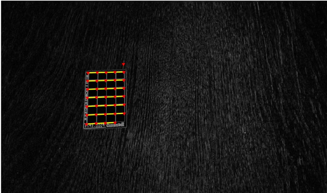
Figure 7: Result of the Lattice Detection algorithm. Lattice Points (red) on a grid (yellow) were detected. The detected points may be coarse, not complete, or incorrect.
